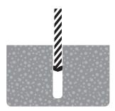
Drill a 20mm hole (Y-Cutter drill bit recommended) to the correct embedment, this should be no more than 80% of the base material thickness.
